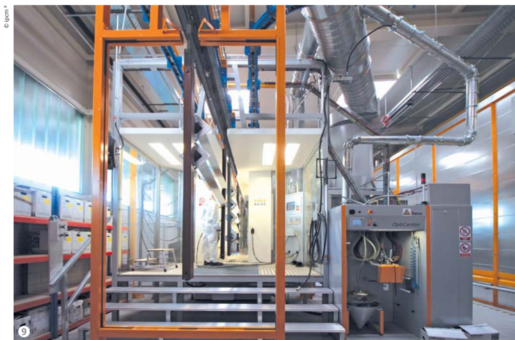
Figure 9: The fast colour change coating booth, with the powder centre on the left, is equipped with 10 automatic guns, all supplied by Gema.
