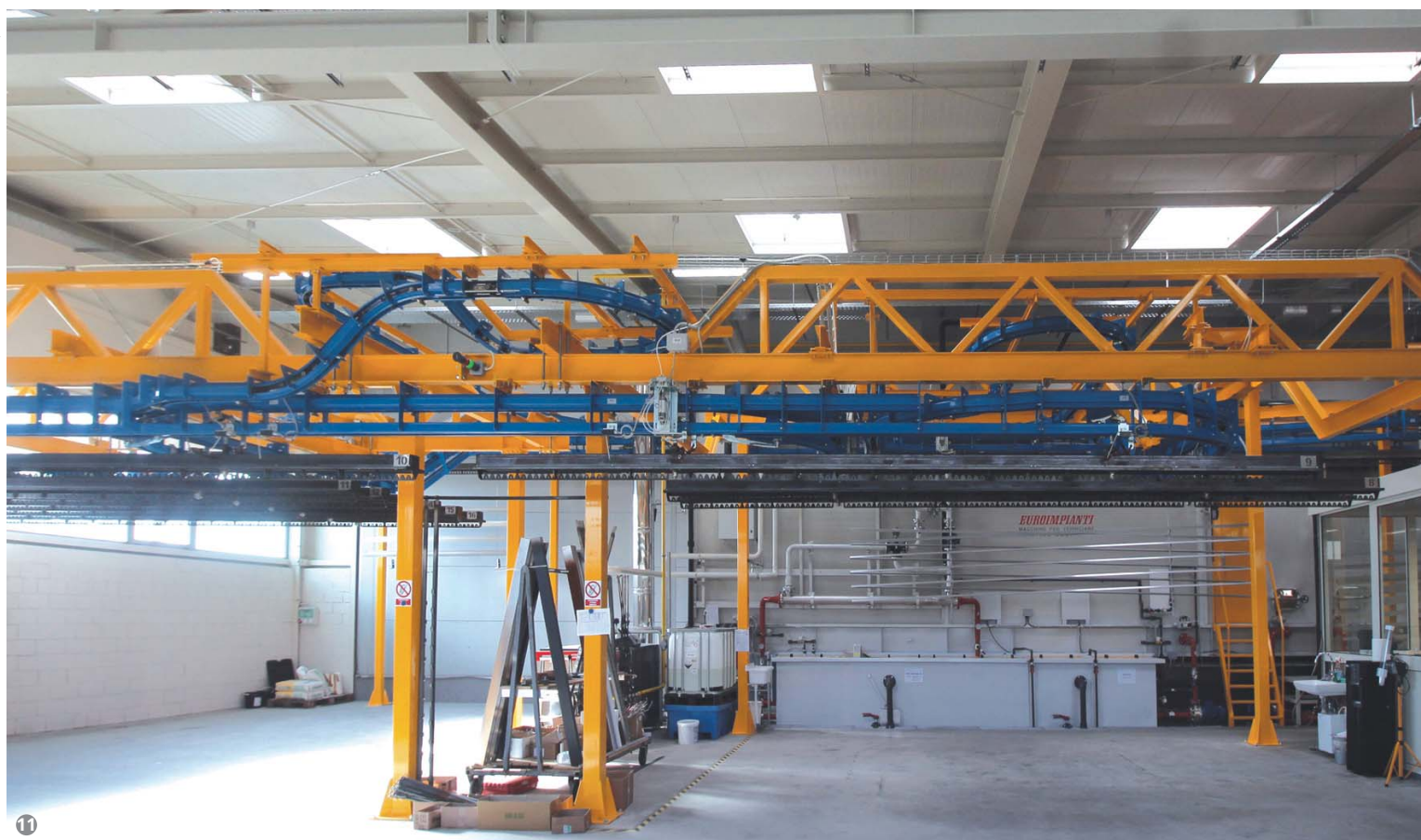
Figure 11: The loading area with the storage buffer before the pre-treatment tunnel.
