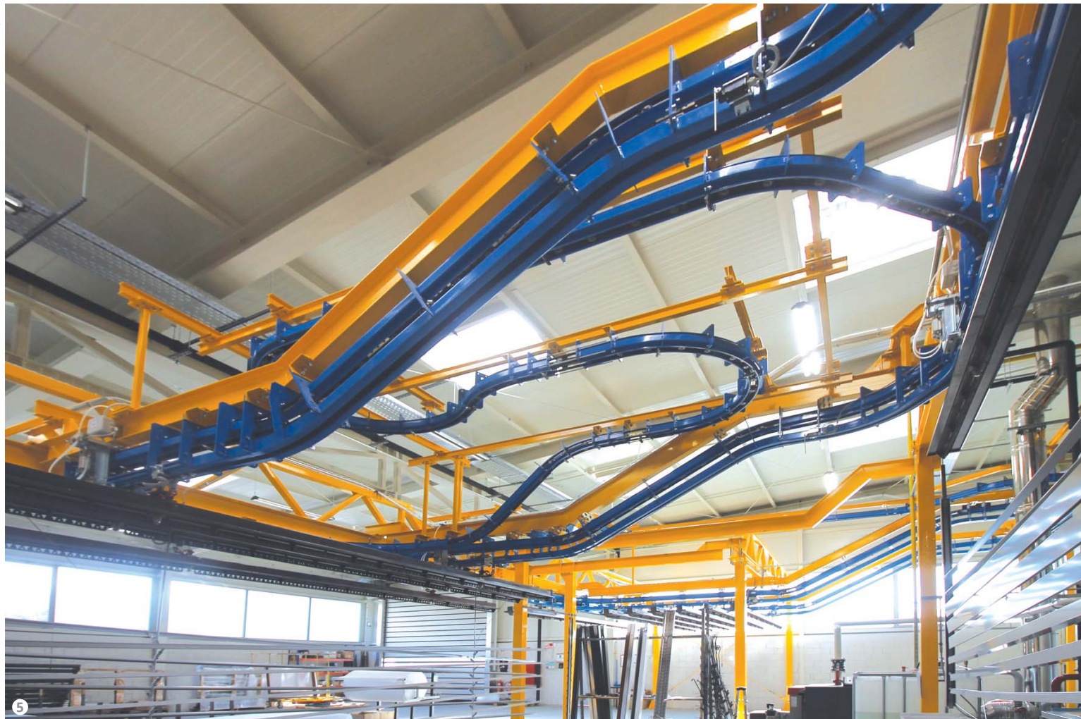
Figure 5: The power&free conveyor supplied by Futura Convogliatori Aerei of Robecco Pavese (Pavia, Italy).
