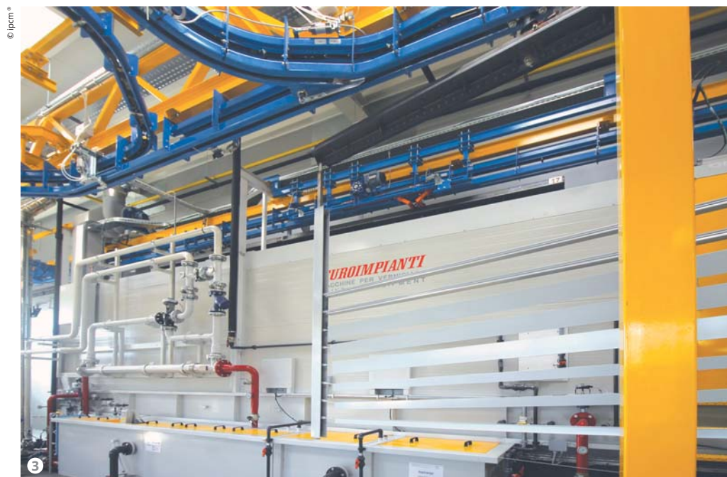
Figure 3: The 7-stage pre-treatment tunnel.
