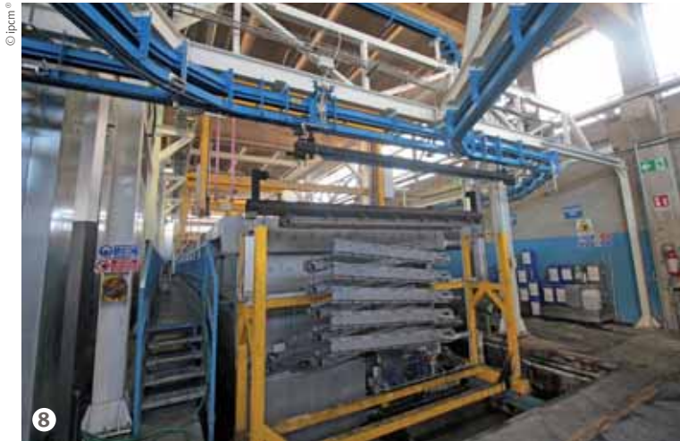
Figure 8: The loading bars are automatically transferred from the conveyor to the bridge crane used for the pre-treatment and cataphoresis tanks.
