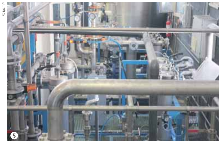
Figure 5: All the main parts of the cataphoresis plant are mounted on two skids.
