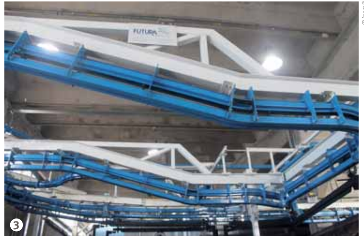
Figure 3: The Power & Free conveyor was provided by Futura Convogliatori Aerei from Robecco Pavese (PV, Italy).
