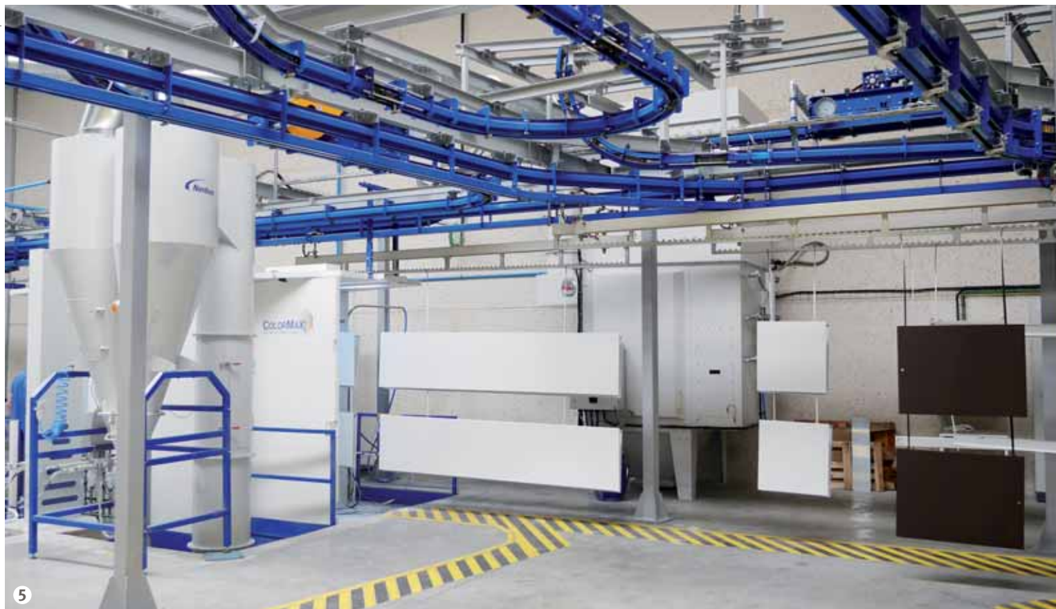
Figure 5: With the new layout, it is possible to paint two colours simultaneously, or apply one colour in a booth and change colour in the other. Any colour can be painted at any time with total flexibility.
