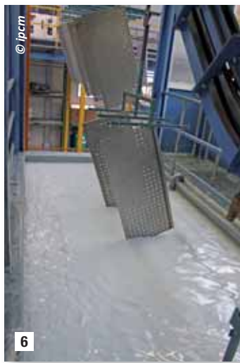
6 Parts immersed in the cataphoresis finishing bath with a two-component acrylic product.
