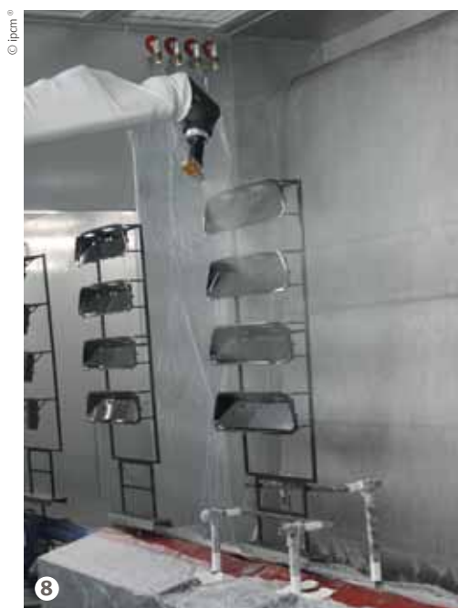
Figure 8: The clearcoat application booth.
