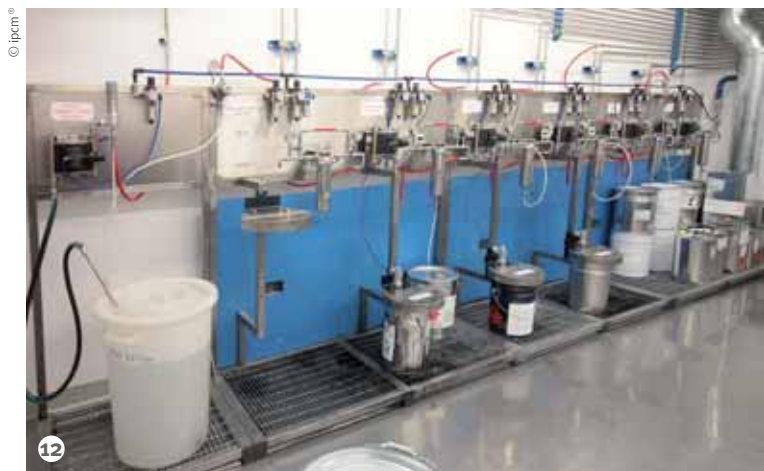
Figure 12: The coating management unit.
