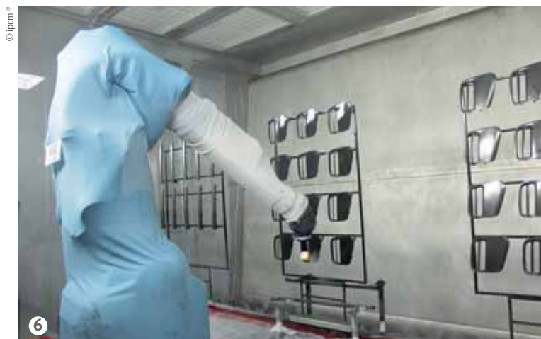
Figure 6: The primer application booth.
