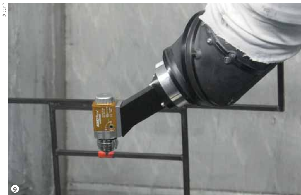
Figure 9: A detail of the paint application with a DeVilbiss pneumatic gun.
