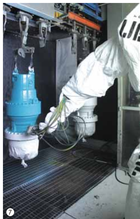
Figure 7: The robotic application of the topcoat.
