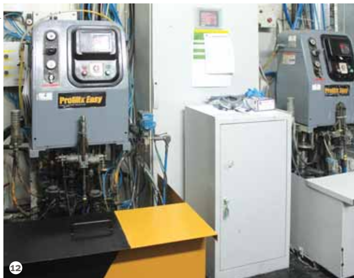
Figure 12: The Promix Easy system for dosing the primer.
