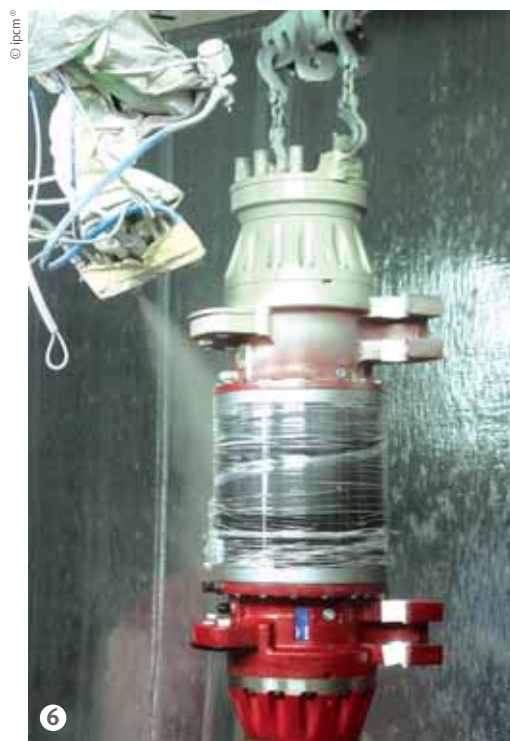
Figure 6: The robotic application of the primer.
