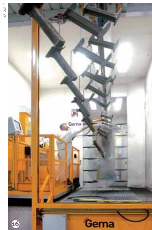
Figure 16: The post-retouching station after the powder application booth.
