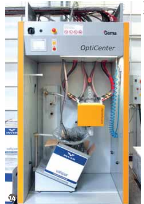
Figure 14: Gema Europe's OptiCenter powder management unit with powders supplied by Inver-Valspar.
