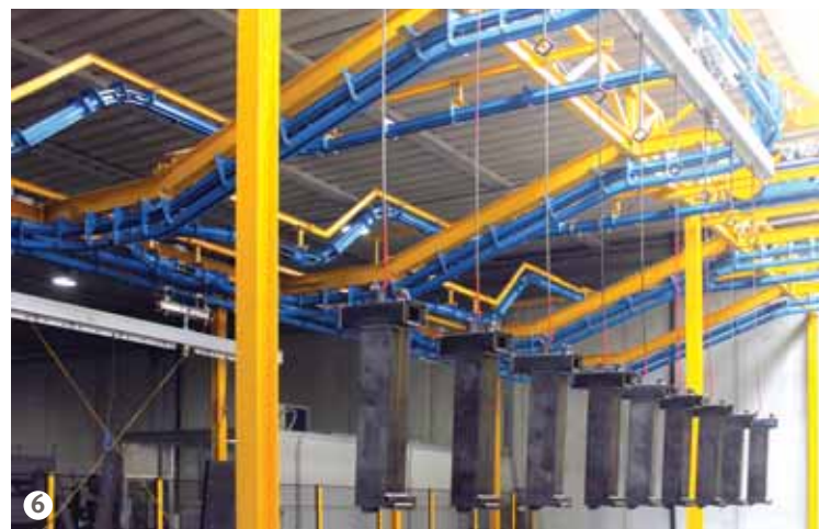
Figure 6: The storage buffer preceding the pre-treatment process.
