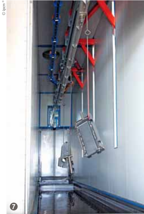
Figure 7: The first pre-treatment stage is an immersion alkaline degreasing process.
