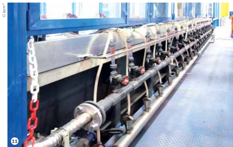
Figure 11: The outside of the cataphoresis tank.
