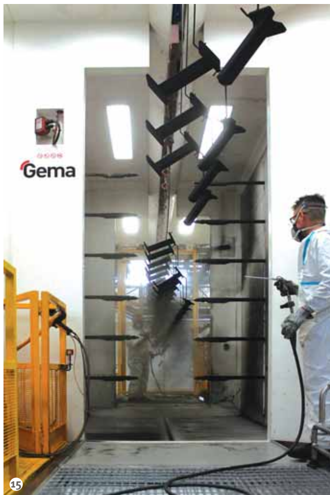
Figure 15: The manual pre-retouching operation.
