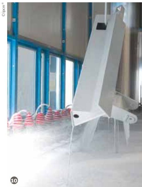
Figure 10: The cataphoresis tank and, in the background, the dialysis cells.
