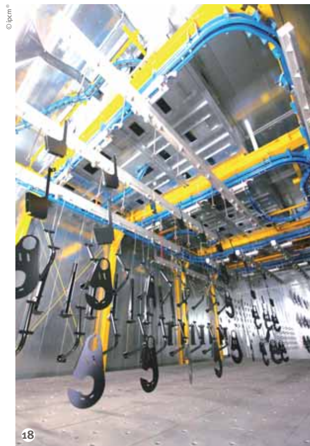
Figure 18: The cooling area for the treated components.
