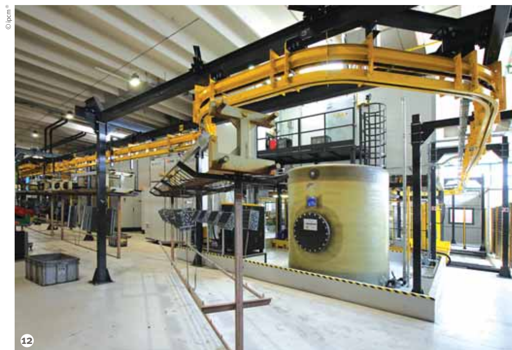
Figure 12: In the foreground, the wastewater treatment tank and, beside it, the evaporator. On top, the Futura Convogliatori Aerei Power & Free conveyor and, in the background, the traverser taking the workpieces to the oven’s monorail conveyor.
