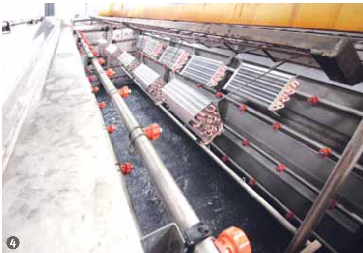
Figure 4: The spray cleaning process with demineralised water.
