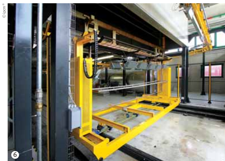
Figure 6: The traverser for transferring the parts to the monorail conveyor of the cataphoresis curing oven.
