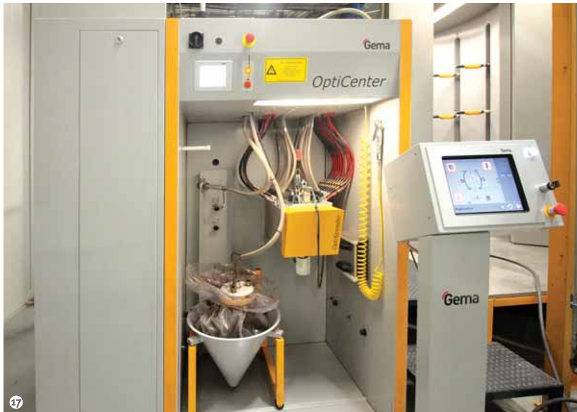
Figure 17: The booths have 16 guns each and use the conventional Venturi powder feeding technology.
