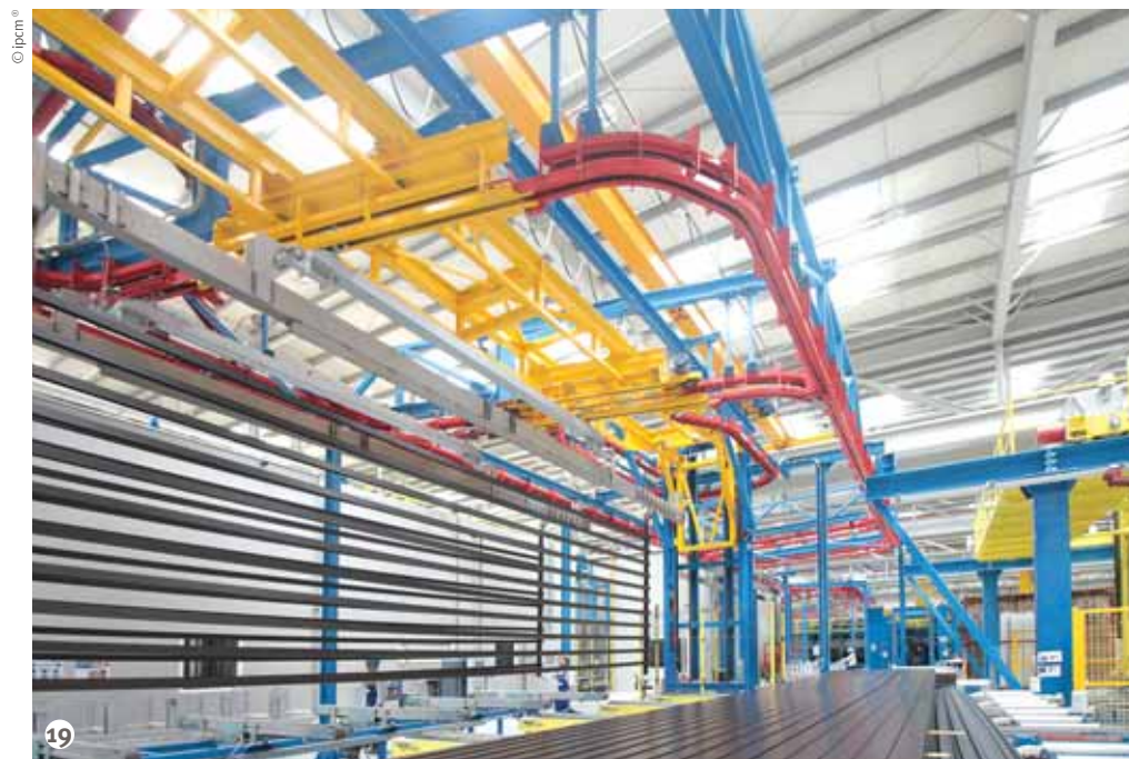
Figure 19: The profile unloading station is in line with the packaging machine.
