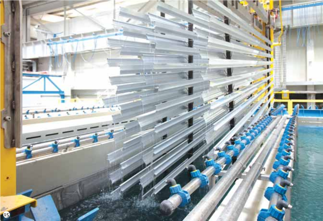
Figure 15: The immersion pre-treatment line can handle 3 bars at a time to ensure the highest possible productivity.
