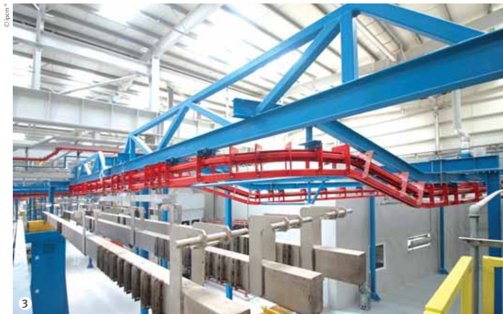
Figure 3: The power & free conveyor designed and built by Futura Convogliatori Aerei has a net load capacity of 500 kg.
