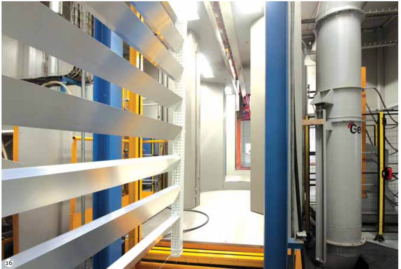
Figure 16: For the powder application, TALEX chose two Magic Cylinder booths with a quick colour change system, supplied by Gema Europe.
