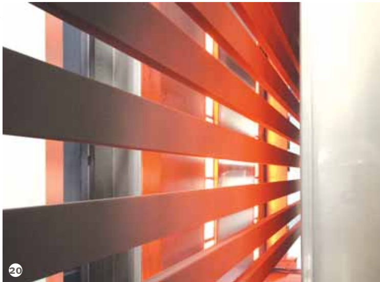
Figure 20: The IR station is used to gel the applied powders and avoid any possible contamination among different shades inside the oven.
