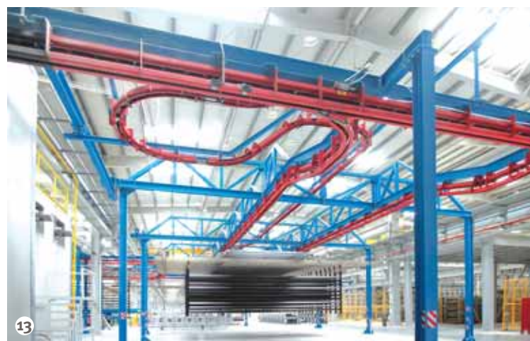
Figure 13: One of the storage buffers created along the conveyor to avoid any loss of productivity.
