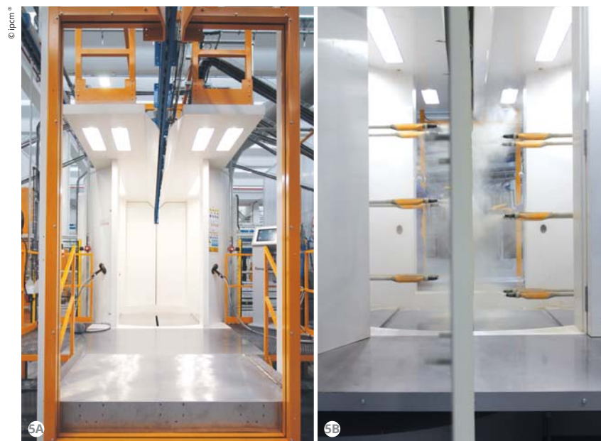
Figures 5A and 5B: The new Gema MagicCylinder coating booth with a quick colour change system
