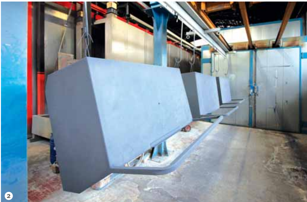
Figure 2: Besides the in-line system, the factory is equipped with a static plant to treat large-sized components.
