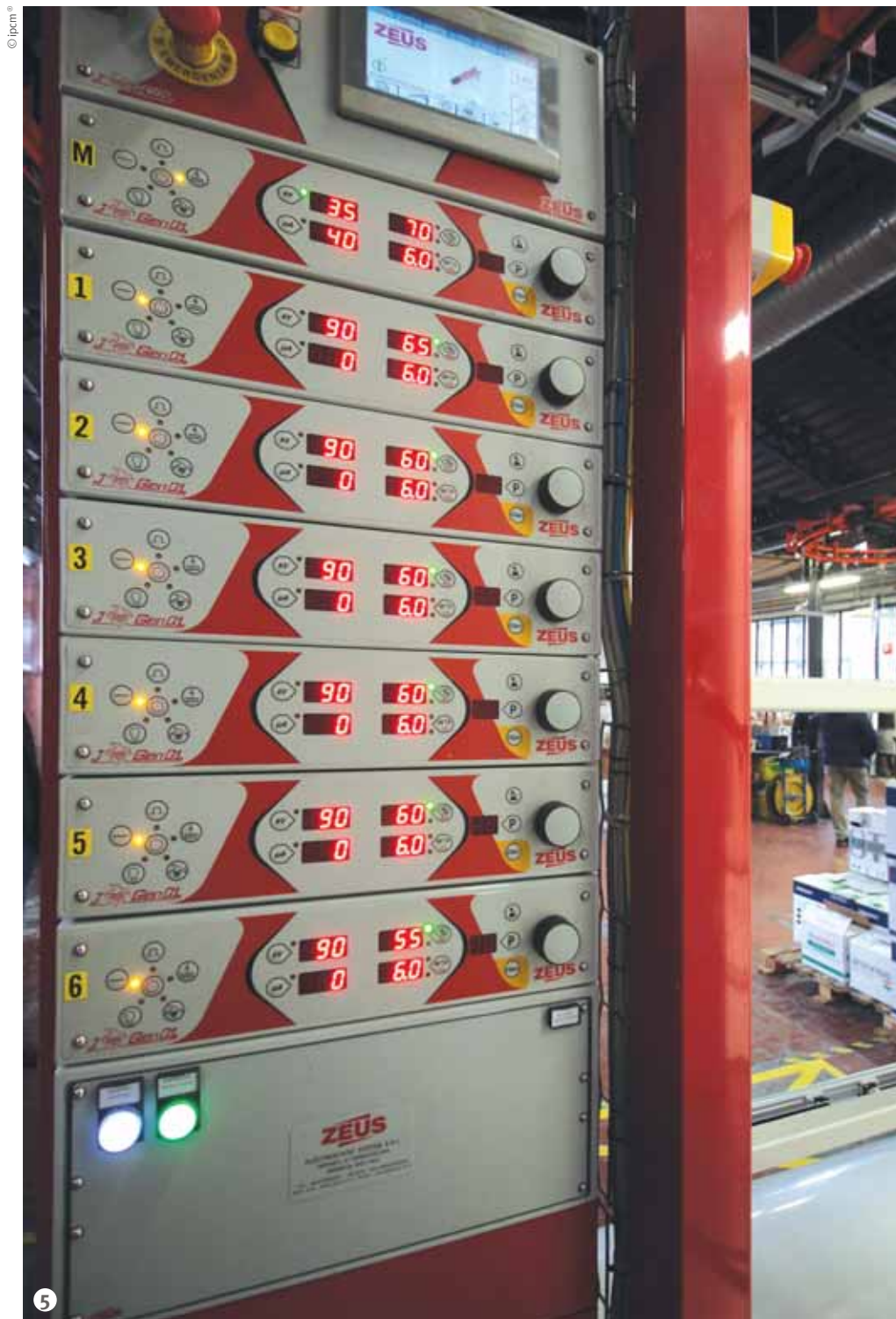
Figure 5: The control modules of the 6 automatic guns and of the manual one.
