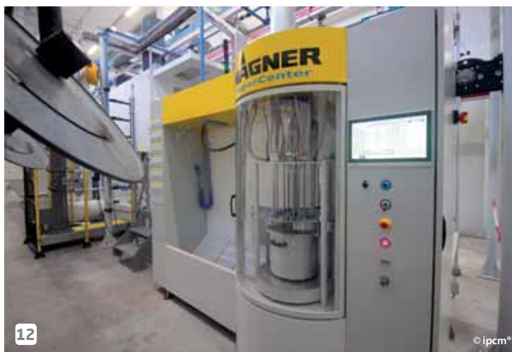
12 The brand new "SuperCenter" powder unit by Wagner Spa the powder coating system is equipped with.
